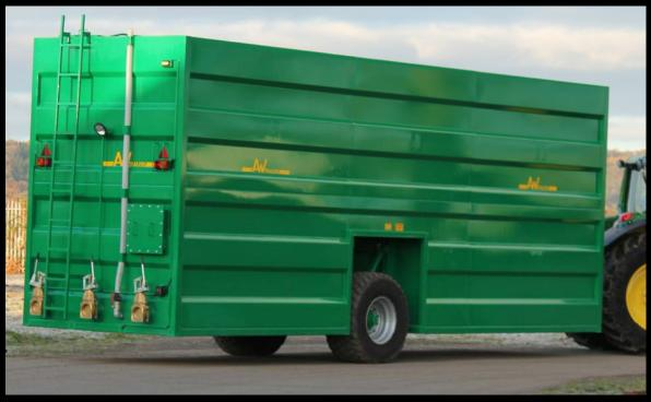
The AW Nursery Tank has a 10 stud commercial hydraulic lifting axle which enables the tank to be lowered flat on to the ground when in position. Standard features include inspection steps, hatches, hydraulic brakes and full road lighting. The standard model has a cubic capacity of 70 cubic metres.
